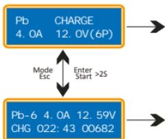
As you can see on left, you can set up the charge current on the left. The nominal of the second line and voltage of the battery on the right of the second line. The charge current ranges from 0.1-10.0A and the voltage should be matched with the battery being charged. Start the charge process by pressing <sup>Enter</sup> <sub>Start</sub> key for more than 2 seconds.
