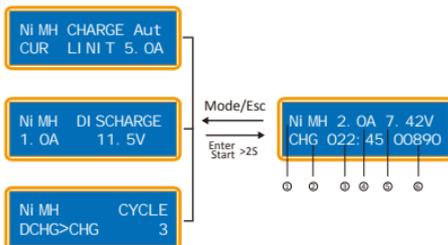
The screen displays the present state of process. To stop It press <sup>Mode</sup> <sub>Esc</sub> key;
