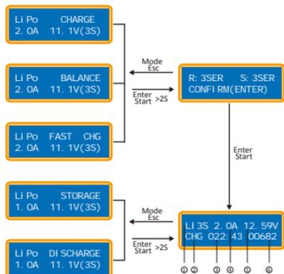
This screen shows the number of cells you set up and the processor detects. “R” shows the number of cells selected by you at the previous menu. If both numbers are identical you can start charging by press **Enter** **Start** button. If not, press **Mode** **Esc** button to go back to previous menu, and then carefully check the number of cells of the battery pack to charge again. If you selected the AUTO mode or discharge mode, you can pass over this screen directly.
